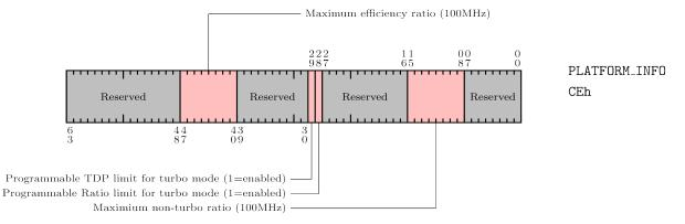
• MSR\_PLATFORM\_INFO Maximum Efficiency Ratio is the only guaranteed frequency regardless of workload.
