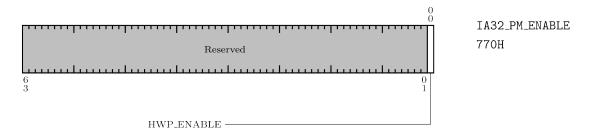
• IA32\_PM\_ENABLE will disable IA32\_PERF\_CTL. The enable bit is sticky and requires a reset to clear.
